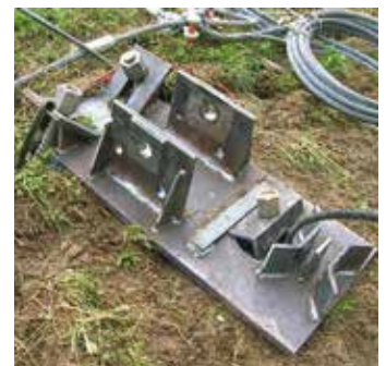
3D verankerbare Bodenplatte 3D anchorable ground plate
